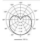
Polar Pattern Measured at 1000 Hz
