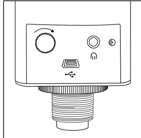
Where your DAW has adequately low latency and you wish to hear some plug-in effects while recording, use your DAW's software monitoring facility and set the microphone balance control to fully DAW only. You can then adjust the mix of what you hear within your DAW in the usual way.
