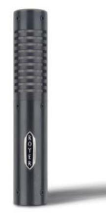
ohms at 1 kHz. Royer recommends using a preamplifier with an input impedance of at least 1,500 ohms for the best results. If the preamp's impedance is too low, the microphone will tend to lose low end and body. Like the SF-12, the SF-1 has a frequency response of 30 Hz to 15 kHz (+/-3 dB) and a sensitivity of -52 dBV per Pascal +/- 1 dB.
