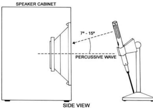
*Slight off-axis positioning will minimize stressing the ribbon on loud sound sources*
