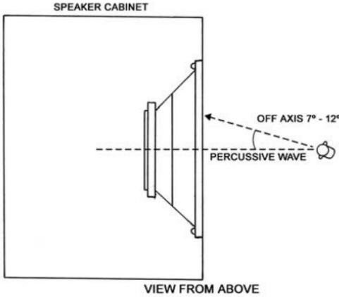
Angling the microphone slightly will minimize stressing the ribbon. Due to the microphone's pick-up pattern, sound will not be affected
