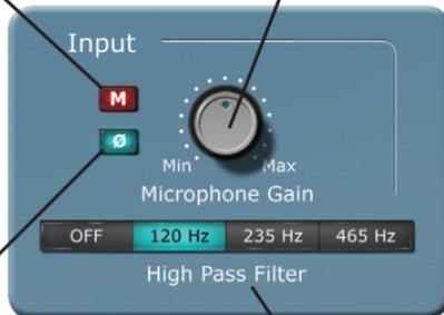
**Phase Invert:** Inverts the phase of the microphone input by 180°
