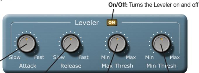
**Attack:** Adjusts the length of time it takes for the input signal to be reduced to the target level after the signal level goes above the **Max Threshold**.
