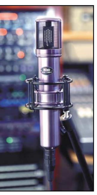
microphone itself, the PPU01 power unit, and some (PC only) software. The DM1001 microphone houses a rectangular dual diaphragm capsule. This rectangular shape is something of a Milab signature that also features in some of the company's more traditional offerings. The idea is that by not using a more conventional circular shape, diaphragm resonances can be more 'naturally' tuned across the response of the microphone.
