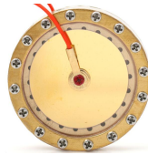
Center Terminated Single Backplate Concentric Holes
