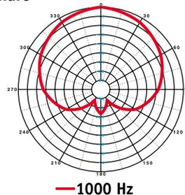
The frequency response chart (above) and the polar patterns represent a typical production run for this microphone.
