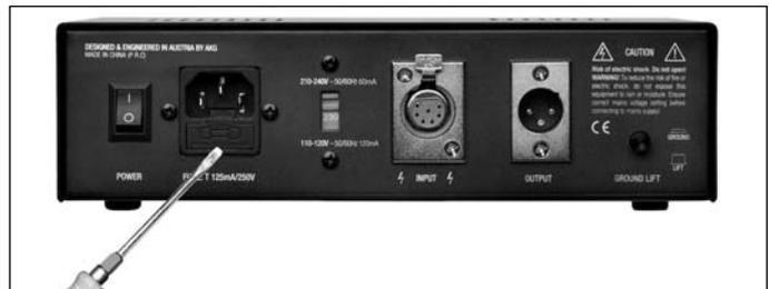
Fig. 20: Opening the fuse compartment.
